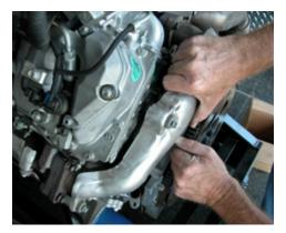
Step 1: Remove shielding from stock up-pipes
