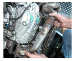
Step 3: Remove left and right stock up-pipes.
