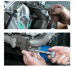
Step 4: Using stock bolts and new PPE Gaskets, install PPE Up-Pipes on driver and passenger sides.
