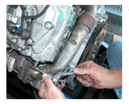
Step 2: Remove bolts from top and bottom flanges on both left and right stock up-pipes. Save bolts for reinstallation.
