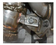
Step 5: Install Down Pipe Bracket.
